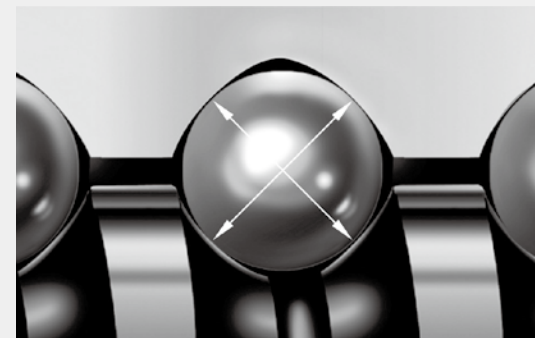
(Contact between ball and Circular-arc Groove)
