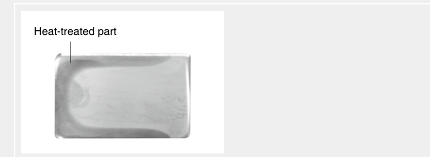
[Fig2. Hardness pattern for flat rail]
